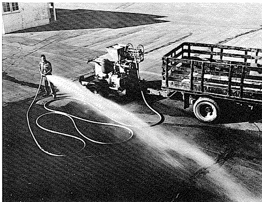
Figure 15. Slip-on tanker-mixer designed and built by Arcadia Equipment Development Center (1961).
